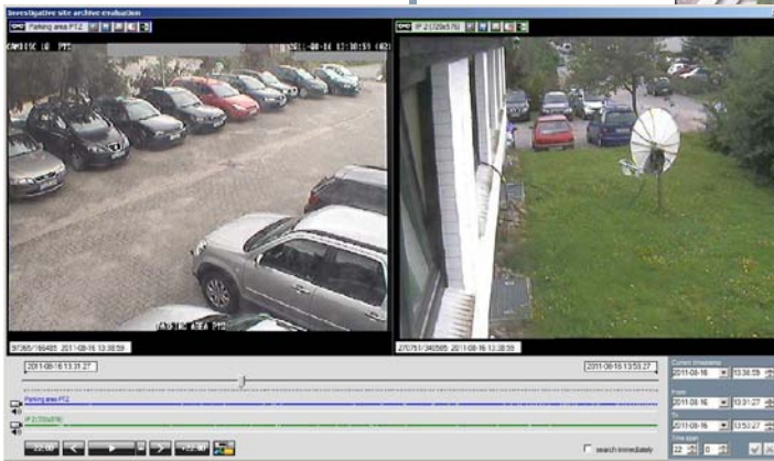
The investigative site archive evaluation allows timesynchronous display and export of the recorded image and audio data of up to two cameras simultaneously.
