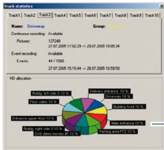
Track statistics with information e.g. on the storage space occupied by each camera track
